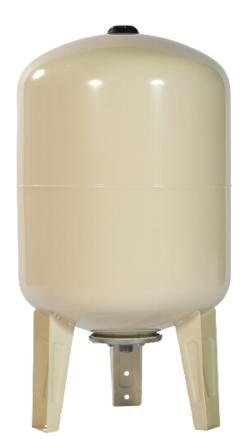
pressurized water in a booster pump system. The pressure tank effectively releases its stored volume of pressurised water on demand and prevents pump start-ups for demands lower than its storage capacity.
